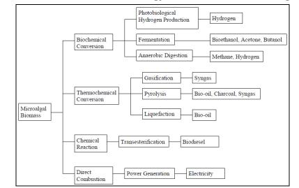
Figure 5. Conversion Processes for Energy Production from Microalgal Biomass
