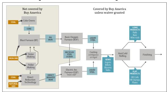
Figure 1. The Iron and Steel Manufacturing Process
